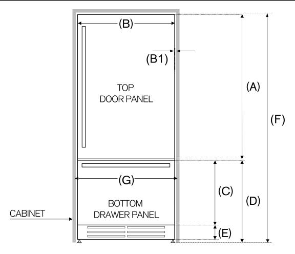
NOTE: The refrigerator comes with a 4" (102 mm) stainless steel toe kick installed to fit a standard 84" (2134 mm) tall cabinet niche. For different toe kick heights, adjust C and D accordingly. For flush installation in a standard 25" (635 mm) deep cabinet niche, maximum custom door panels thickness is 15/16" (24 mm).
